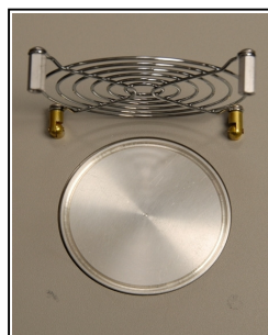
Top-loading Hot-Plate with protective flip-up heat shield, simply set film samples on top of hot-plate for shrinkage testing (Shown at left). Easy-to-read backlit measurement grid for measuring shrinkage of samples after removing from hot-plate (Shown above).
